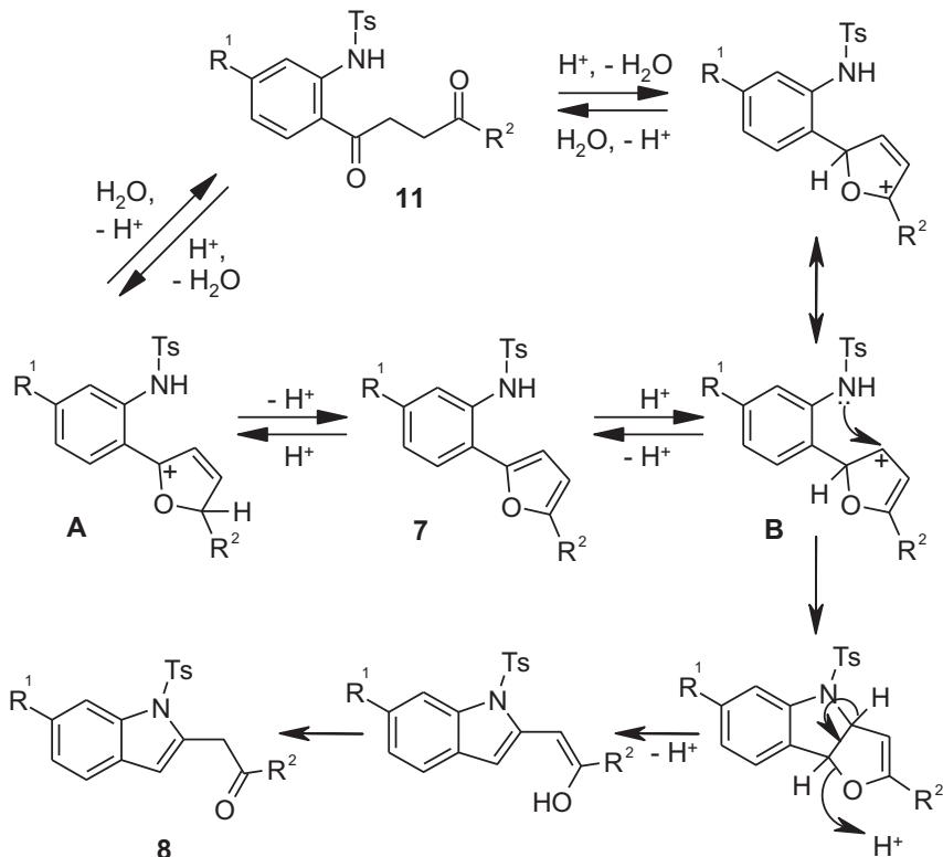
**Scheme 2.** Plausible mechanism for recyclization of arylfurans **7**.
