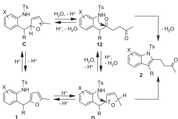
**Scheme 3.** The proposed mechanism for recyclization of benzylfurans **1**.
