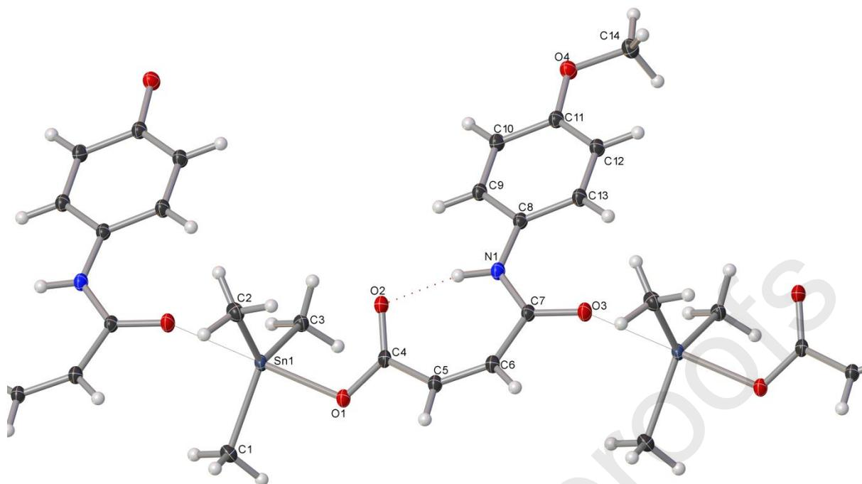
**Figure 1.** A perspective of one of the linear polymeric chains of compound **1**. The displacement ellipsoids are drawn at the 50% probability level and H atoms are shown as small circles of arbitrary radii.
