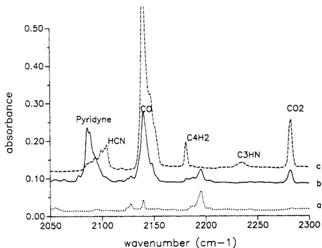
**Figure 1.** IR spectra of 3,4-PDA and its photolyzed products in the 2050–2300-cm<sup>-1</sup> region in an N<sub>2</sub> matrix at 13 K: (a) 3,4-PDA; (b) after 100 min photolysis through water and λ > 340-nm filter (The peak at 2281 cm<sup>-1</sup> is due to <sup>13</sup>CO<sub>2</sub>); (c) following additional 30 min photolysis with λ > 210 nm.
