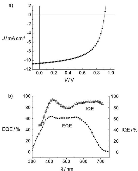
**Figure 2.** a)  $J$ - $V$  curve of a PBDTTBT/PC<sub>70</sub>BM-based solar cell device under illumination of AM1.5G, 100 mWcm<sup>-2</sup>. b) External quantum efficiency (EQE) and internal quantum efficiency (IQE) of a PBDTTBT/PC<sub>70</sub>BM-based solar cell device.
