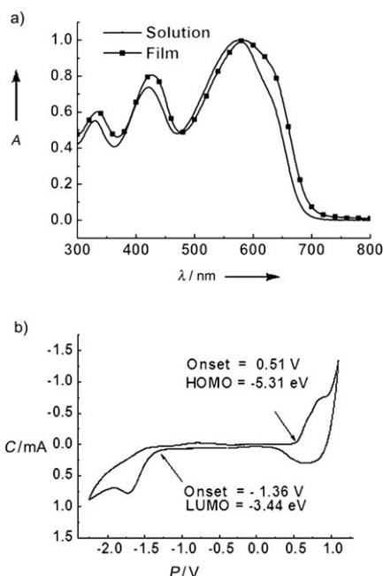
**Figure 1.** a) Absorption spectra of PBDTTBT as a film and in chloroform solution. b) Cyclic voltammograms of PBDTTBT films on a platinum electrode in  $0.1 \text{ mol L}^{-1}$  Bu<sub>4</sub>NPF<sub>6</sub>, CH<sub>3</sub>CN solution.
