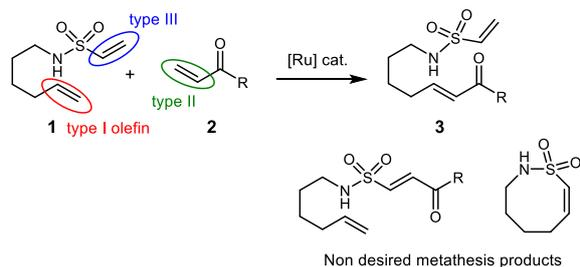
**Scheme 2.** Classification of olefins and plausible metathesis reactions between substrates **1** and **2**.
