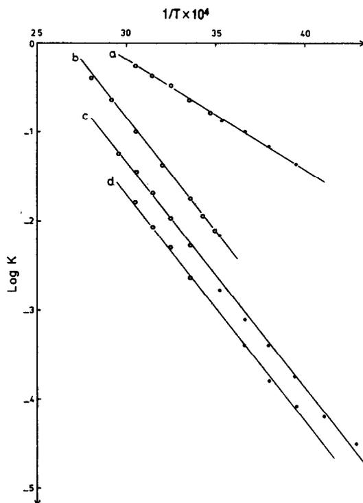
Fig. 3. Plots of the logarithm of the equilibrium constants  $K$  versus the reciprocal of temperature ( $1/T$ ), in chloroform (a), 1,4-dioxane (b), tetrahydrofuran (c), acetone (d) by measurement of line intensities in the absence of exchange ( $\bullet$ ) or from the coalesced spectra ( $\circ$ ).
