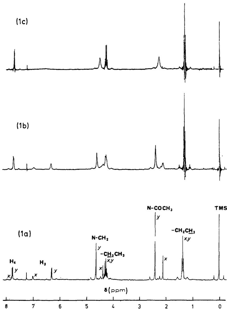
Fig. 1. The spectrum of compound (1) at  $-10^\circ\text{C}$  (1a),  $25^\circ\text{C}$  (1b) and  $55^\circ\text{C}$  (1c) at 250 MHz in  $\text{CDCl}_3$ .
