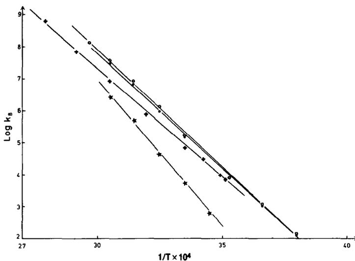
Fig. 5. Arrhenius plots of rate constants  $k_\beta$  (or  $k_\alpha$ ) in the four solvents used: chloroform ( $\star$ ), 1,4-dioxane (+), tetrahydrofuran (O), and acetone ( $\bullet$ ).
