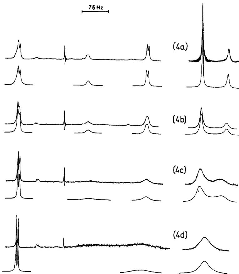
Fig. 4. Experimental and theoretical curves (above and below respectively) for the exchange of the methylic protons of the amide group (right) and the ring protons  $H_3$ ,  $H_4$  (left) as a function of the temperature: 15°C (4a), 25°C (4b) 35°C (4c), 45°C (4d).
