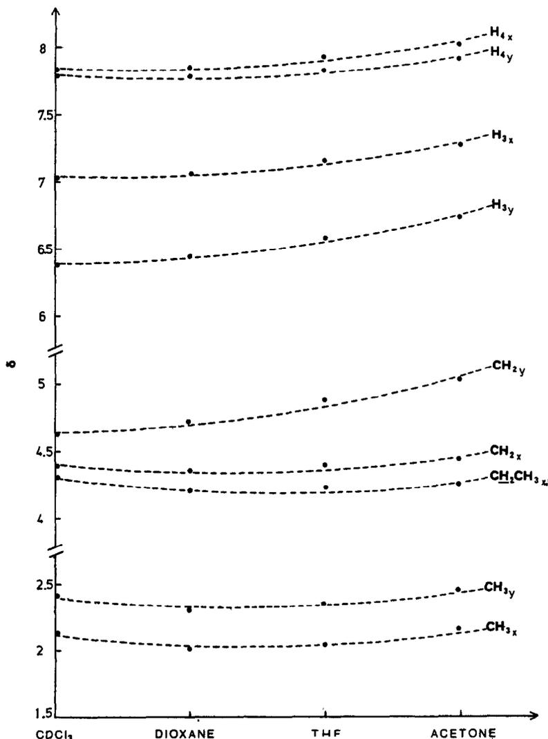
Fig. 6. Graph of chemical shifts (in ppm from TMS) for the protons of compound (1) as a function of the solvent.
