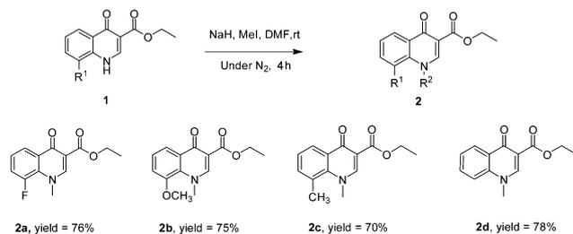
**Scheme 2** Synthesis of *N*-methylated derivatives **2** from compound **1**. *Reaction conditions:* compound **1** (1 mmol), NaH (0.036 mg, 1.5 mmol), MeI (0.284 g, 2 mmol) in DMF at 60 °C. Stirring under N<sub>2</sub> atmosphere, 4 h. Isolated yields after column chromatography.
