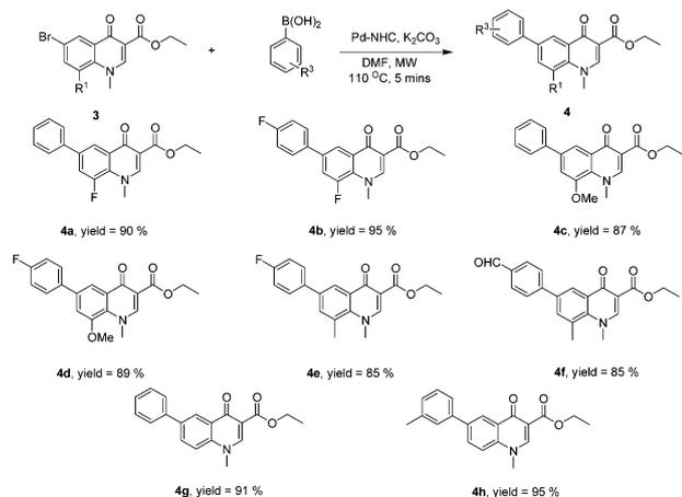
**Scheme 4** Synthesis of 6-aryl-4-quinolones. *Reaction conditions:* compound **3** (1 mmol), aryl boronic acid (1.2 mmol), K<sub>2</sub>CO<sub>3</sub> (2 mmol), Pd-NHC (0.0192 g, 2 mol%), dry DMF (3 mL), Microwave, 110 °C, 5 min. Isolated yields after column chromatography purification.
