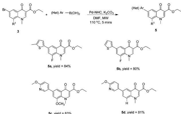
**Scheme 5** Suzuki cross coupling with heteroarylboronic acids forming products **5**. *Reaction conditions:* compound **3** (1 mmol), heteroarylboronic acid (1.2 mmol), K<sub>2</sub>CO<sub>3</sub> (2 mmol), Pd-NHC (0.0192 g, 2 mol%), DMF (3 mL), microwave, 110 °C, 5 min. Isolated yields after column chromatography purification.
