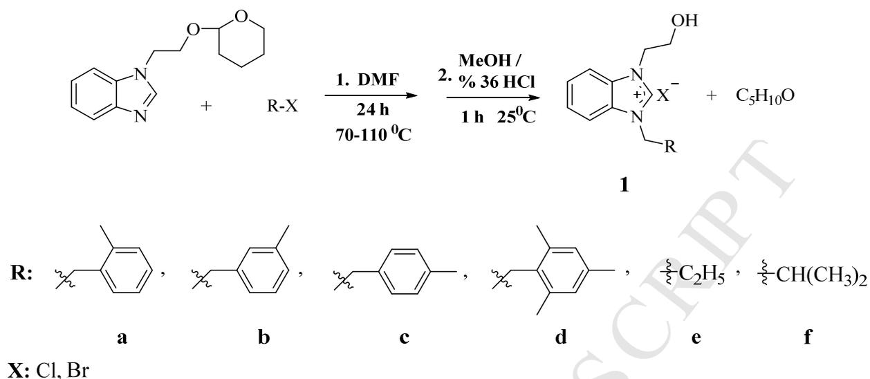
**Scheme 1.** Synthesis of 2-hydroxyethyl substituted NHC precursor **1a-f**
