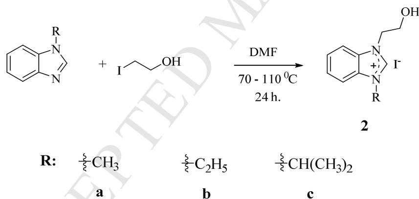
**Scheme 2.** Synthesis of 2-hydroxyethyl substituted NHC precursor **2a-c**
