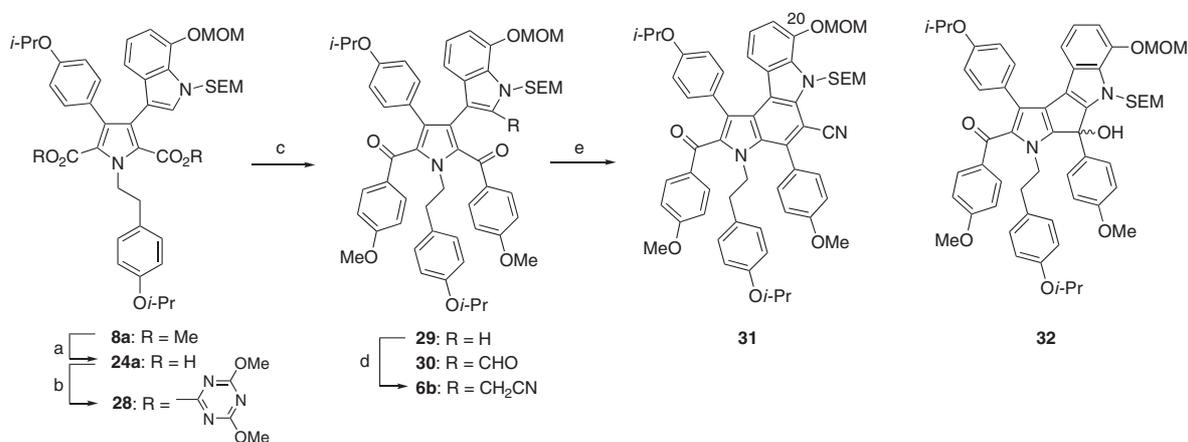
**Scheme 5.** Construction of the Core Pyrrolo[2,3-c]carbazole System of Dictyodendrin B.
