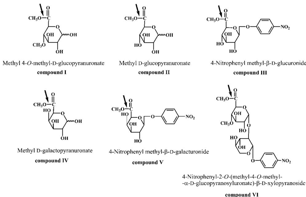
**Fig. 1.** Synthetic Substrates for Determination of GE Activity by TLC (compound I), HPLC (compound VI) and by the Hestrin Procedure (compounds I–V).
