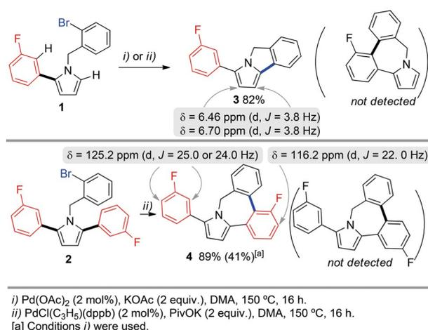
**Scheme 1.** Palladium-catalyzed direct cyclization reactions of 1-(2-bromobenzyl)-2-(3-fluorophenyl)pyrrole and 1-(2-bromobenzyl)-2,5-bis(3-fluorophenyl)pyrrole. DMA: *N,N*-dimethylacetamide; dppb: 1,1'-bis(diphenylphosphanyl)butane; Piv: pivaloyl.
