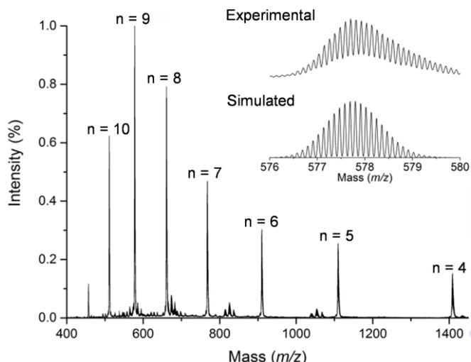
**Figure 6.** HR-ESI-TOF mass spectrum of  $[\text{Pd}_6(\mathbf{2a})_8](\text{BF}_4)_{12}$  showing signals due to  $[\text{Pd}_6(\mathbf{2a})_8(\text{BF}_4)_{12-n}]^{n+}$ ,  $n = 4 - 10$ . Inset: comparison of experimental (top) and simulated (bottom) spectra for the signal of  $[\text{Pd}_6(\mathbf{2a})_8(\text{BF}_4)_3]^{9+}$  ( $m/z = 577.705$ ).
