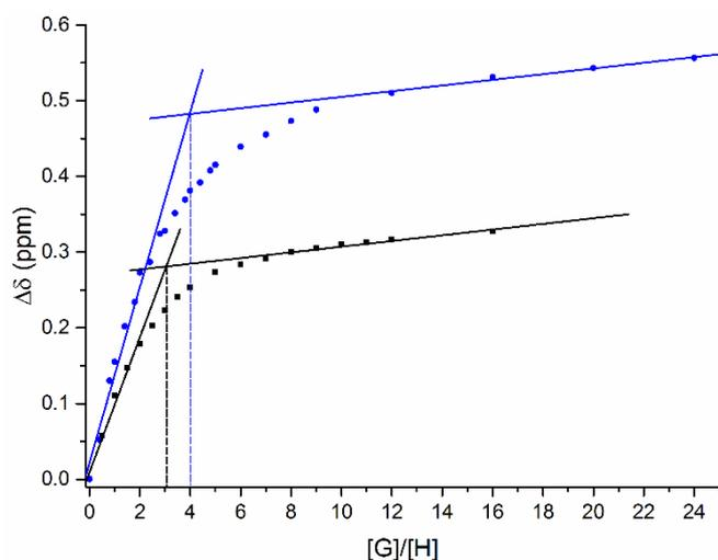
**Figure 7.** Mole-ratio titration plots (500 MHz, *d*<sub>6</sub>-DMSO, 298 K)<sup>[28]</sup> showing the <sup>1</sup>H chemical shift change of the internally directed proton H<sub>6</sub> of the [Pd<sub>6</sub>(**2a**)<sub>8</sub>]<sup>12+</sup> (blue data) and [Pd<sub>6</sub>(**1a**)<sub>8</sub>]<sup>12+</sup> (black data) cages with increasing equiv. of TsO<sup>-</sup> guest (from 0 to 22 equiv.). [Host] = 1.07 mM.
