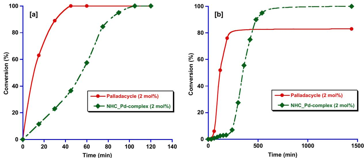
**Fig. 2.** Conversions versus the time for the coupling reaction of 2-bromonaphthalene with the diethyl vinylphosphonate using the Herrmann palladacycle (●) or the (NHC) palladium complex (◆) at 140 °C ([a]) or 110 °C ([b]). Reaction conditions: 3 mmol 2-bromonaphthalene, 3 mmol diethyl vinylphosphonate, 2 mol% [Pd], 3 mmol K<sub>2</sub>CO<sub>3</sub>, 30 mL DMF.
