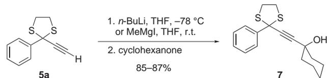
**Equation 3** Reaction of **5a** with a carbonyl compound
