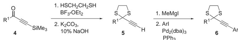
**Equation 2** Two-step synthesis of substituted propargylic dithioacetal **6****Table 1** Synthesis of Propargylic Dithioacetals from **4**
