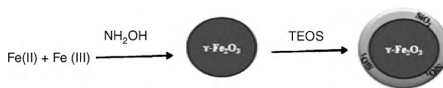
Fig. 1. Schematic synthesis of \gamma\text{-Fe}_2\text{O}_3@SiO_2 .
