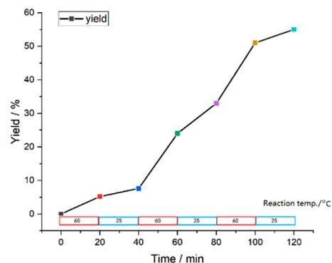
**Figure 2.** “On–off” experiment: tracking of the yields for different reaction times with heating turned on or off every 20 min. All of the yields were determined by <sup>1</sup>H NMR spectroscopy using mesitylene as the internal standard.
