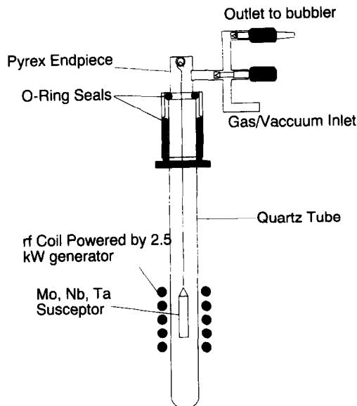
Fig. 2. Glass reaction vessel for preparation of samples by inductive heating.
