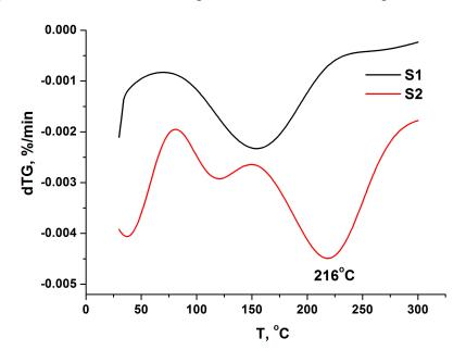
Figure 1. Derivative of thermogravimetric curves for samples S1 and S2.
