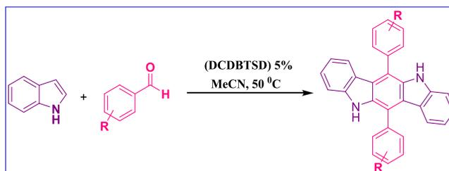
**Figure 2.** The synthesis of 6,12-disubstituted 5,7-dihydroindolo [3,2-*b*]carbazoles. [Color figure can be viewed at wileyonlinelibrary.com]
