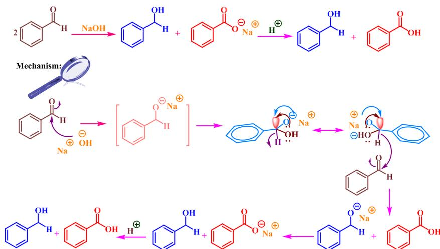
**Figure 4.** The proposed mechanism for the *in situ* oxidation–reduction in Cannizzaro reaction through unusual hydride transfer via anomer-based oxidation [26]. [Color figure can be viewed at wileyonlinelibrary.com]
