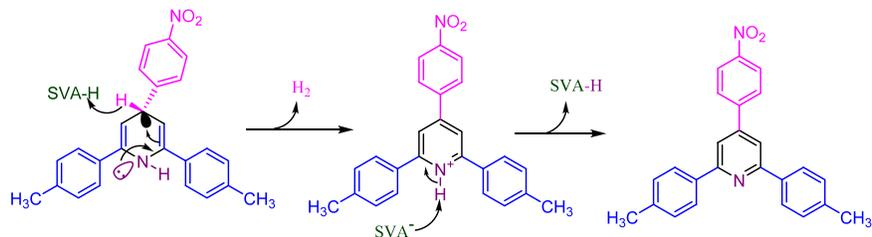
**Figure 7.** The synthesis of 2,4,6-triarylpyridines through anomeric-based oxidation [29]. [Color figure can be viewed at [wileyonlinelibrary.com](http://wileyonlinelibrary.com)]
