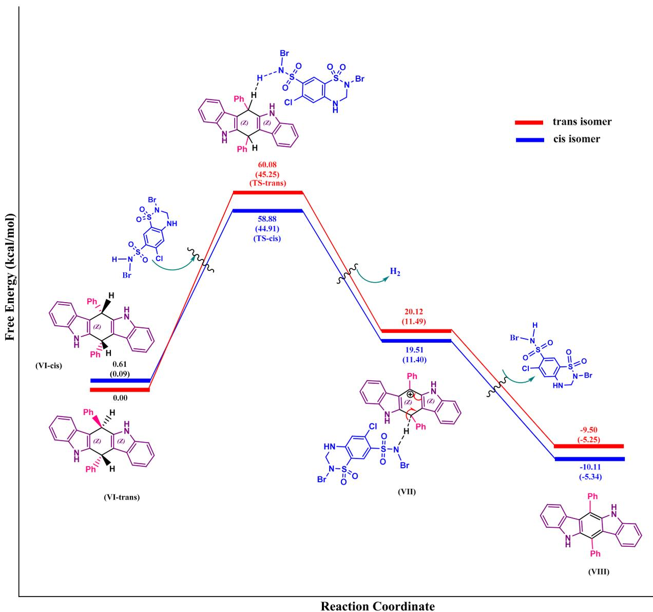
**Figure 8.** Energy profile calculated for synthesis of indolo[3,2-b]carbazole by catalyst DCDBTSD beginning from compound VI (see Fig. 3). The relative Gibbs-free energies in acetonitrile and the gas phase total electronic energies ( $E_{el} + ZPE$ , figures in parentheses) obtained from the B3LYP/SVP calculations both are given in kcal/mol. [Color figure can be viewed at [wileyonlinelibrary.com](http://wileyonlinelibrary.com)]
