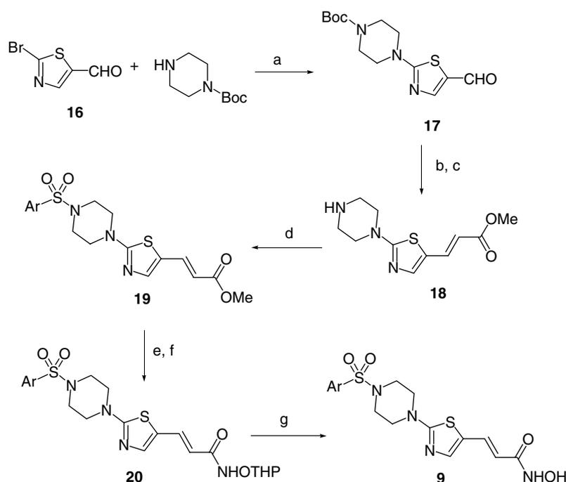
**Scheme 3.** Reagents and conditions: (a) K<sub>2</sub>CO<sub>3</sub>, MeCN, 80 °C, 8 h (92%); (b) trimethylphosphonoacetate, *n*-BuLi, THF, -50 °C, 2 h (74%); (c) 4 M HCl/dioxane, 2 h (97%); (d) arylsulfonyl chlorides, Et<sub>3</sub>N, DCM, rt, 4–12 h (86%); (e) NaOH, MeOH, rt, 5 h (95%); (f) HN<sub>2</sub>OHP, EDCI, HOBT, Et<sub>3</sub>N, DCM, rt, 12 h (83%); (g) HCl, MeOH, Et<sub>2</sub>O, rt, 5 h (91%).
