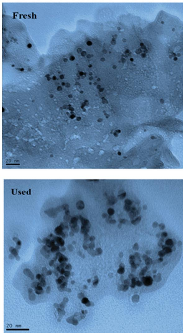
Fig. 4 Transmission electron micrographs of fresh and used (after 4th cycle) NAP-Mg-Pd(0) catalysts.
