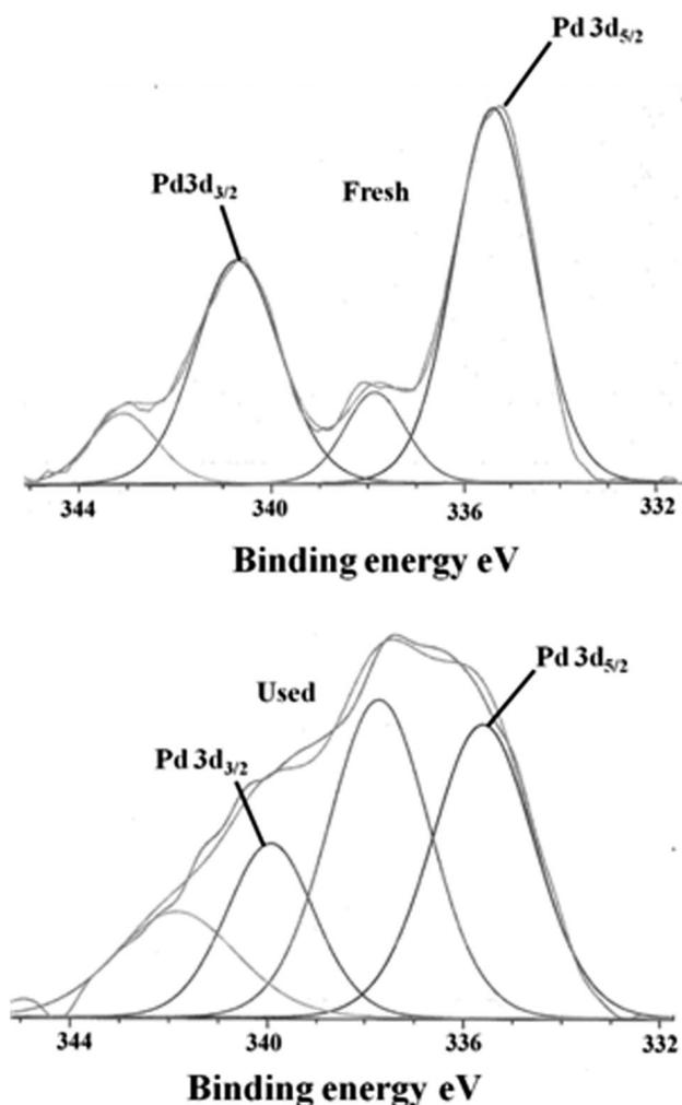
Fig. 2 X-ray photoelectron spectra of fresh and used NAP-Mg-Pd(0) catalysts.
