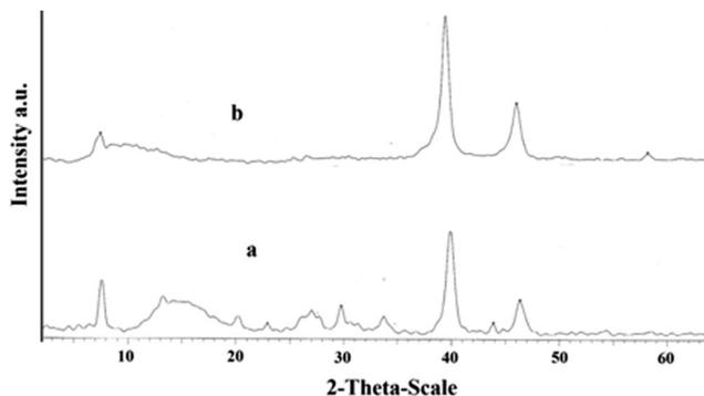
Fig. 1 XRD patterns of the fresh (a) and used (b) NAP-Mg-Pd(0) catalysts.
