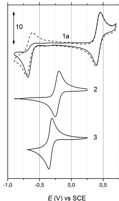
**Figure 3.** Cyclic voltammograms of radicals 1a, 2, and 3 (400 μM) in phosphate buffer (0.1 M, pH 7.4, containing 0.1 mM EDTA) at 0.02 V·s<sup>-1</sup> (solid line) and 0.5 V·s<sup>-1</sup> (dashed line). Intensities (ordinate, in μA) were divided by the square root of the scan rate to allow direct comparisons.
