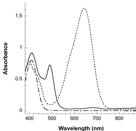
**Figure 4.** UV-vis spectra of radical **2** (solid line), its anion  $2^-$  (dotted line), and triarylmethane **2-H** (dashed line). Triaryl anion  $2^-$  was formed by the reduction of radical **2** ( $50 \mu\text{M}$  **2** in  $0.1 \text{ M}$  phosphate buffer at  $\text{pH}$  7.4 containing  $0.1 \text{ mM}$  EDTA) with an excess of sodium dithionite.
