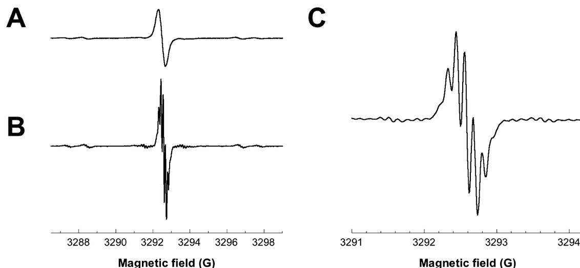
**Figure 2.** EPR spectrum of radical 3 in phosphate buffer (0.1 M, pH 7.4) in the presence of O<sub>2</sub> (A) or in the absence of O<sub>2</sub> (B). Enlargement of the spectrum recorded under anaerobic conditions to observe the hyperfine structure (C).
