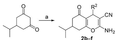
**Scheme 3.** Synthesis of **2b–f** starting from commercially available 5-isopropylcyclohexa-1,3-dione and the appropriate commercially available aldehyde R<sup>2</sup>CHO, by use of a one-pot three-component reaction. *Reagents and conditions:* a) malononitrile, appropriate commercial aldehyde (R<sup>2</sup>CHO), amine base, EtOH, RT (22–62 %).
