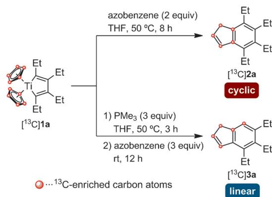
**Scheme 4.** <sup>13</sup>C-Labeling experiment for the formation of indenenes **2a** and **3a**.
