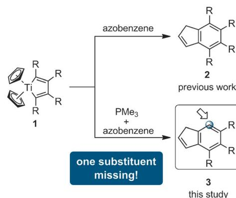
Scheme 1. Novel C–C bond-cleavage reaction of a titanocene.
