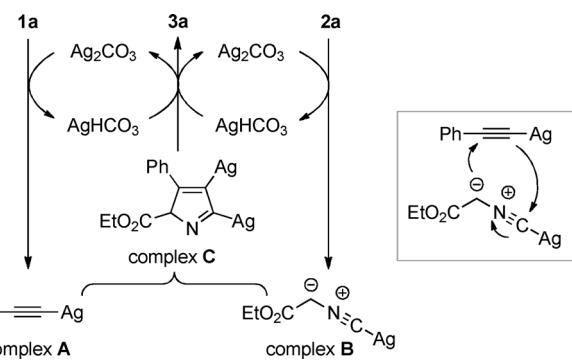
**Scheme 4.** Proposed mechanism for the silver-catalyzed cycloaddition of terminal alkynes with isocyanides.
