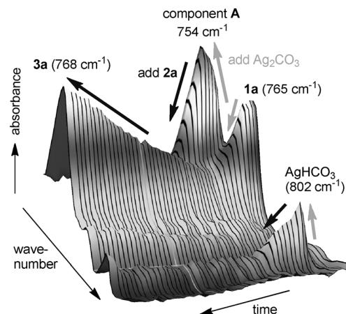
**Figure 1.** Profile of the stepwise stoichiometric reaction between **1a**, Ag<sub>2</sub>CO<sub>3</sub>, and **2a** in DMSO at 80 °C monitored by *in situ* IR spectroscopy.
