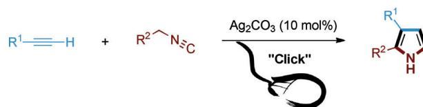
**Just click with silver:** Pyrroles are prepared by the co-cyclization of terminal alkynes and isocyanides in a silver-catalyzed click reaction. This protocol represents an extremely simple, efficient, and
