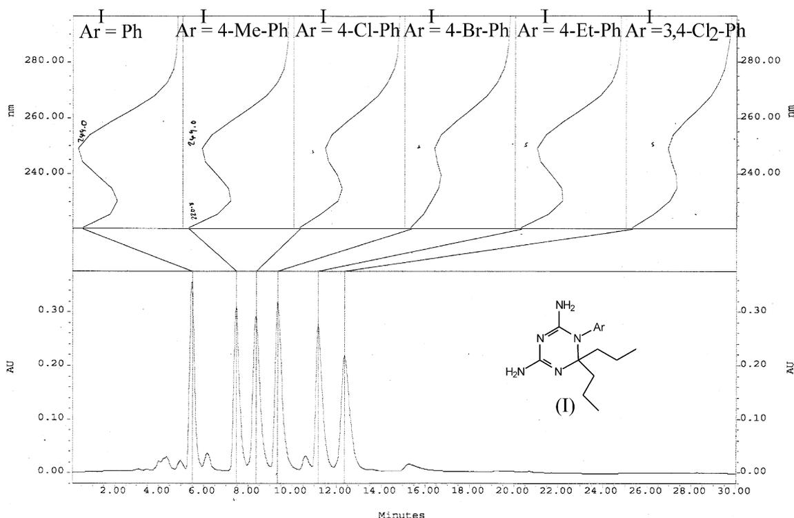
**Figure 1.** HPLC data of **I-11(a-f)**. Column: Hypersil™ 5  $\mu$ m BDS C<sub>18</sub> (4.6 $\times$ 250 mm); Mobile phase: 0.1 M triethylammonium acetate (pH 7.0):acetonitrile gradient from 15–60% over a period of 15 min with an equilibration period of 5 min; UV-detector at 254 nm.
