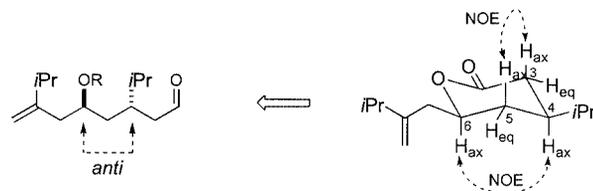
Scheme 2. Determination of the relative configuration.
