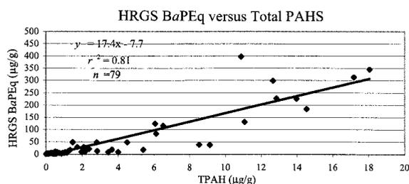
Fig. 5. Correlation between human reporter gene system (HRGS) benzo[*a*]pyrene equivalents (BaPEq) and total polycyclic aromatic hydrocarbons (PAHs). Sample 11 was excluded because of the very high value (1,584) and sample 17 was excluded because of suspect chemical data.
