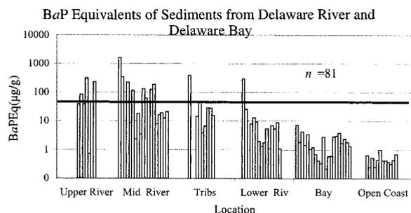
Fig. 2. Distribution of benzo[*a*]pyrene equivalents (*BaPEq*) taken from 81 sediment samples along the Delaware River, Delaware Bay, and Delaware, USA, coast. Categories were based on hydrogeography, salinity, sediment type, and location. Samples exceeding 60  $\mu\text{g BaPEq/g}$  represented by the line would be expected to exhibit degraded benthic communities [9].
