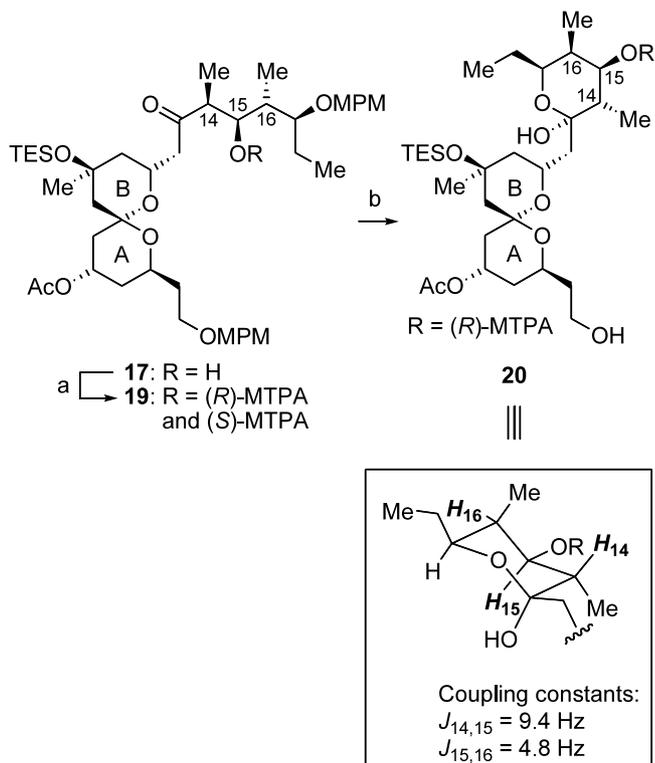
**Scheme 3.** Determination of the C14-16 stereochemistry of **17**. *Reagents and conditions:* (a) (*S*)-(+)-MTPACl or (*R*)-(-)-MTPACl, Et<sub>3</sub>N, DMAP, CH<sub>2</sub>Cl<sub>2</sub>, rt (80%); (b) DDQ, CH<sub>2</sub>Cl<sub>2</sub>-H<sub>2</sub>O, rt (75%). MTPA = 2-methoxy-2-phenyl-2-(trifluoromethyl)acetyl.
