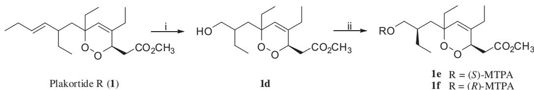
**Fig. 3.** Conversion of plakortide R (**1**) into alcohol **1d** and its MTPA esters **1e** and **1f**. Reagents and conditions: (i) O<sub>3</sub>, CH<sub>2</sub>Cl<sub>2</sub>, –78 °C, 1 min; then NaBH<sub>4</sub>, MeOH, 2 h; (ii) (*R*)- or (*S*)-MTPACl, DMAP/CH<sub>2</sub>Cl<sub>2</sub>, rt, 3 h.
