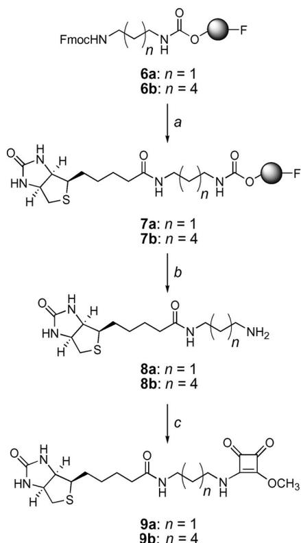
Scheme 2. Synthesis of model compounds **9a** and **9b**. a) i) Piperidine (20% in DMF); ii) HOAt, DIC, D-biotin, DMF; b)  $3 \times$  TFA (90% in  $H_2O$ ), quantitative yield and 70% yield, respectively; c) dimethyl squarate, TEA, DMF, quantitative yield for both **9a** and **9b**.
