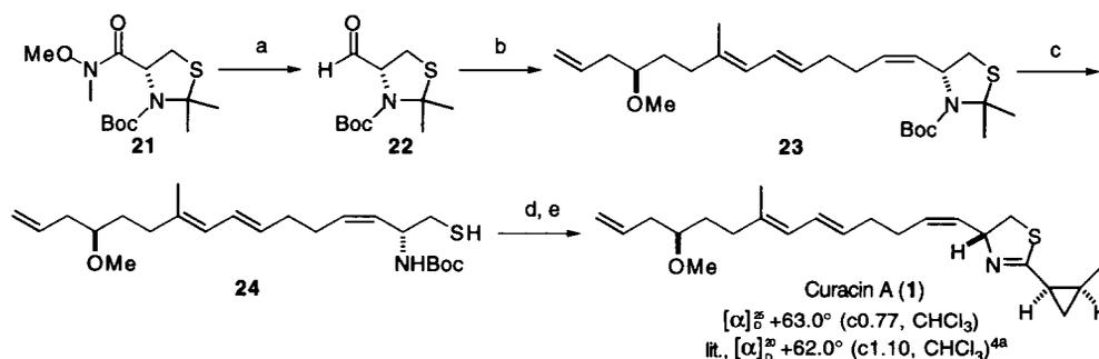
**Reagents and conditions:** (a) LiAlH<sub>4</sub>, ether, 0 °C, 0.5 h (92%); (b) **13**, LiHMDS, THF, -78 °C, 0.5 h, then **22**, THF, -78 °C, 2 h (60% and recovery of **22**, 25%); (c) TFA, CH<sub>2</sub>Cl<sub>2</sub>, 20 °C, 6 h; (d) (-)-**19**, BOPCl, Et<sub>3</sub>N, CH<sub>2</sub>Cl<sub>2</sub>, 20 °C, 3 h; (e) TFA, CH<sub>2</sub>Cl<sub>2</sub>, 20 °C, 2 h, then benzene, reflux, 2.5 h (10% from **23**)
