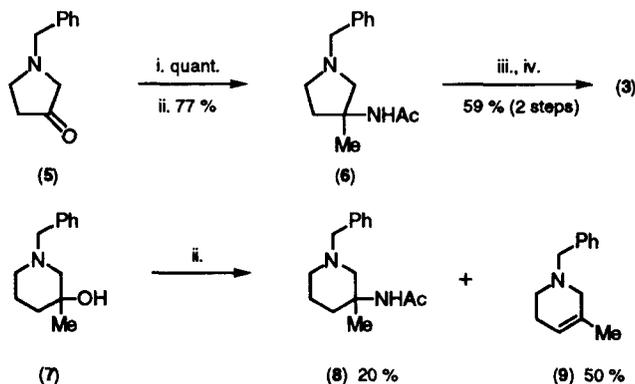
**Reagents and Conditions:** i. MeMgBr, THF-Et<sub>2</sub>O, 0°C; ii. c.H<sub>2</sub>SO<sub>4</sub>, MeCN, 0-5°C; iii. H<sub>2</sub> Pd-C, EtOH, R.T.; iv. Methyl (*R*)-*O*-trifluoromethylsulphonyl lactate, <sup>1</sup>Pr<sub>2</sub>NEt, CH<sub>2</sub>Cl<sub>2</sub>, R.T.
