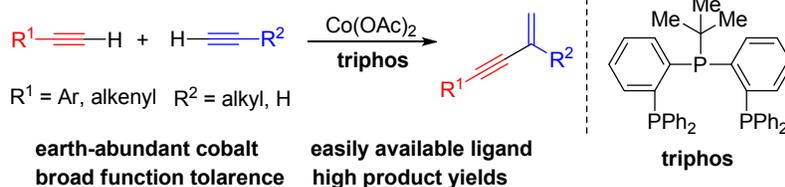
To develop a selective cross-dimerization of two different terminal alkynes, the catalyst has to control three processes in case of metal acetylide mechanism: 1) selective metal-acetylide formation with one of the two terminal alkynes; 2) coordination of metal-acetylide with only the other alkyne to avoid homo-dimerization; 3) regioselectivity in the acceptor alkyne (gem or linear) (Figure 1). During our investigation on the Co(I)-catalyzed enol ester formation between alkynes
