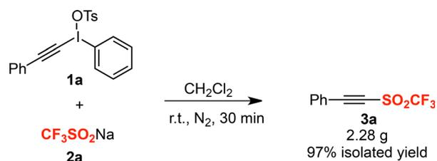
**Scheme 2.** Scaled-up synthesis of **3a** from **1a** and **2a**.
