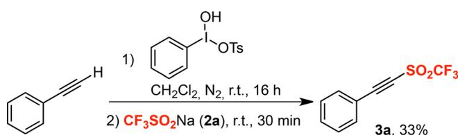
**Scheme 3.** One-pot synthesis of **3a** from ethynylbenzene and **2a**.
