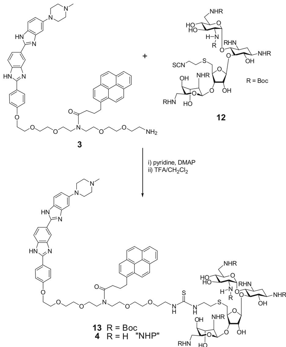
**Scheme 2.** Preparation of triple recognition agent NHP. Reagents and conditions: (i) pyridine, DMAP, 52%; (ii) 1:1 TFA/CH<sub>2</sub>Cl<sub>2</sub>, quantitative.
