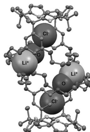
Figure 2. Single-crystal X-ray structures of dimeric complex of receptor **1** ( $[\mathbf{1}\cdot\text{LiCl}(\text{H}_2\text{O})_2]_2$ ). Note that the two crown moieties of chloride-bound receptors hold two lithium ions to form a dimeric hydrated ion-pair complex.
