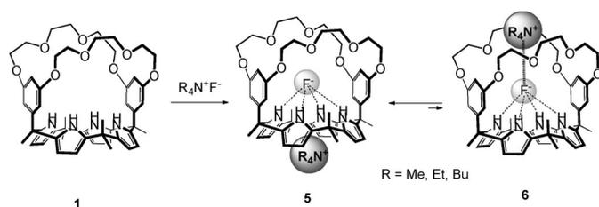
Scheme 2. Proposed binding modes of receptor **1** with tetraalkylammonium fluoride in  $\text{CDCl}_3$ . Receptor-separated ion-pair complex **5** and contact ion-pair complex **6**.
