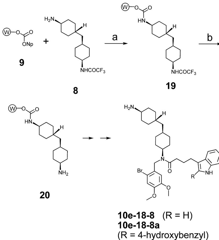
**Scheme 7.** Reagents and conditions: (a) DIEA, DMF, rt, 60 h; (b) NaBH<sub>4</sub>, *n*-BuOH, rt, 49 h; 50 °C, 3 h.
