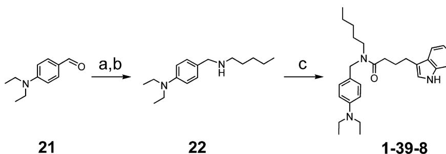
**Scheme 9.** Reagents and conditions: (a) pentylamine, trimethyl orthoformate, rt, 3 days; (b) NaCNBH<sub>3</sub>, 0–5 °C, 2 h; (c) 3-indolebutyric acid, PyBroP, diisopropylethylamine, CH<sub>2</sub>Cl<sub>2</sub>, rt, 1 h.
