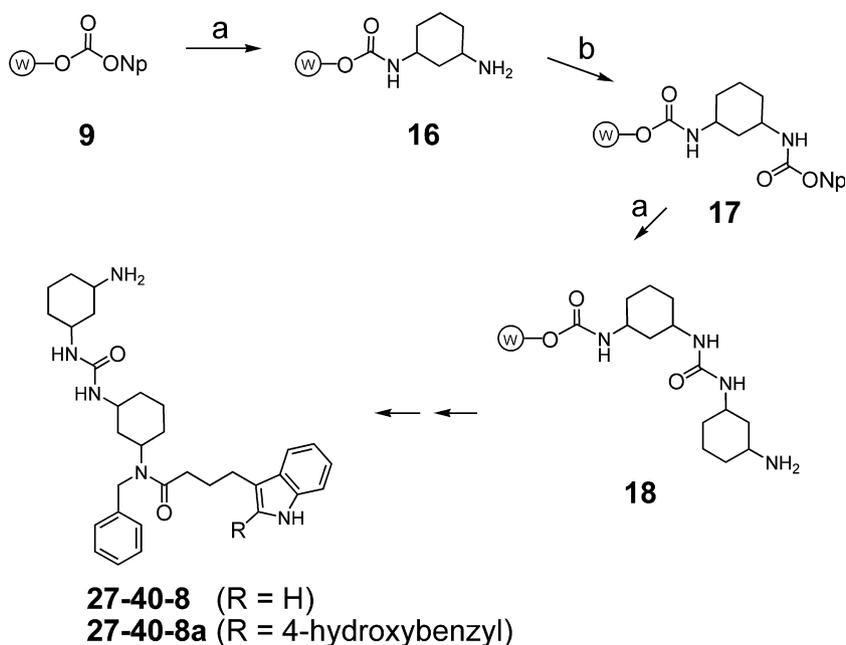
**Scheme 6.** Reagents and conditions: (a) 1,3-diaminocyclohexane, DMF, rt, 24 h; (b) 4-nitrophenylchloroformate, DIEA, DMF, rt, 24 h.
