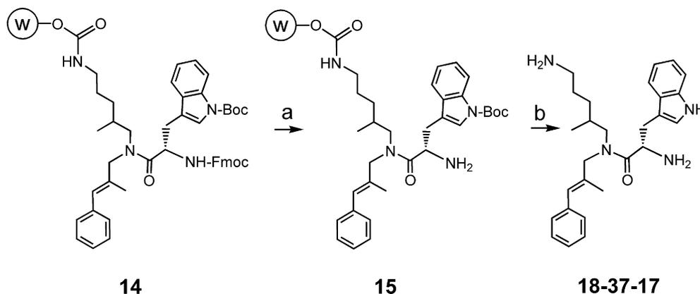
**Scheme 5.** Reagents and conditions: (a) 20% piperidine in DMF, rt, 10 min; (b) trifluoroacetic acid–1,2-ethanedithiol–triisopropylsilane–water (10:2:0.25:0.25), rt, 1 h.
