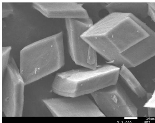
Fig. 1 SEM image of  $\text{Cu}_2(\text{TPTC})$
