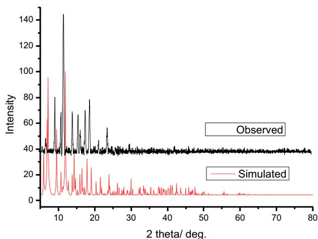
Fig. 2 XRD pattern of  $\text{Cu}_2(\text{TPTC})$
