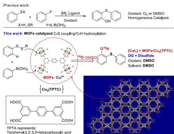
**Scheme 1**  $\text{Cu}_2(\text{TPTC})$  MOF-catalyzed disulfide-directed C–S coupling/ $\text{C}$ –H hydroxylation
