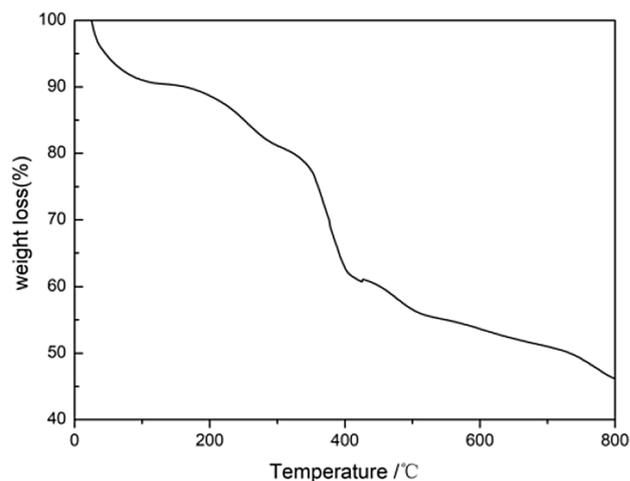
Fig. 3 TGA pattern of  $\text{Cu}_2(\text{TPTC})$
