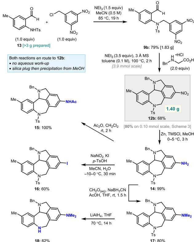
both **9b** and **12b** were purified in this sequence by a single precipitation/trituration from methanol, without the need for an aqueous workup or recourse to conventional silica gel chromatography.
