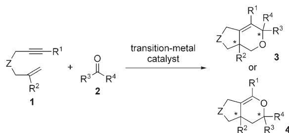
**Scheme 2.** Transition-metal-catalyzed [2+2+2] cycloaddition of 1,6-ynye with ketone.
