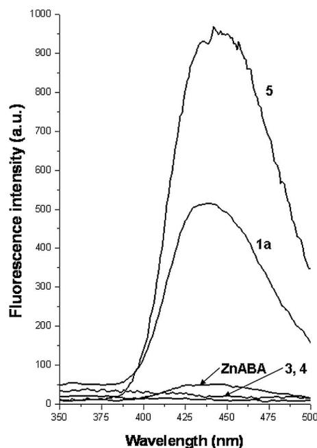
Figure 4. Fluorescence emission spectra of **1a** and **2–5** in aqueous solution (10 μM, 25 mM HEPES buffer, 0.1 M NaClO<sub>4</sub>, pH = 7.4, I = 0.1). All the excitation wavelengths are at 260 nm.
