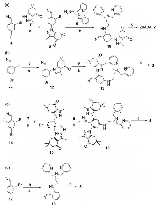
Scheme 1. Synthesis of 2-aminobenzamides. Reagents and conditions: (a) K<sub>2</sub>CO<sub>3</sub>, DMF or NaH, DMF; (b) PdCl<sub>2</sub>, DPPF, NaOtBu, toluene, 100 °C; (c) KOH, H<sub>2</sub>O<sub>2</sub>, EtOH/DMSO.
