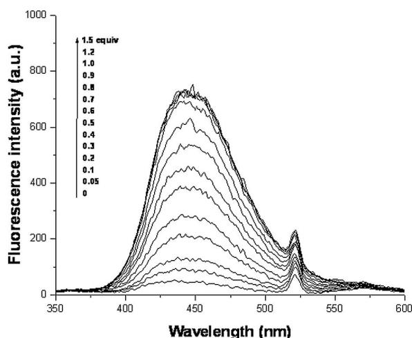
Figure 5. Fluorescence emission spectra (excitation at 260 nm) of ZnABA (10  $\mu$ M; in 25 mM HEPES buffer, 0.1 M NaClO<sub>4</sub>, pH = 7.4,  $I$  = 0.1) upon addition of Zn<sup>2+</sup> [added as Zn(ClO<sub>4</sub>)<sub>2</sub>, 0–15  $\mu$ M]. The small peak at 520 nm arises from second-order scattering.
