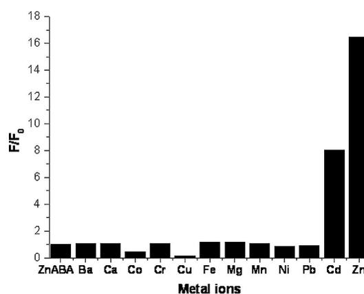
Figure 6. Selectivity of ZnABA towards Zn<sup>2+</sup> and other metal ions. Experimental conditions: ZnABA (10  $\mu$ M; in 25 mM HEPES buffer, 0.1 M NaClO<sub>4</sub>, pH = 7.4,  $I$  = 0.1), 10  $\mu$ M Ba<sup>2+</sup>, Ca<sup>2+</sup>, Co<sup>2+</sup>, Cr<sup>3+</sup>, Cu<sup>2+</sup>, Fe<sup>3+</sup>, Mg<sup>2+</sup>, Mn<sup>2+</sup>, Ni<sup>2+</sup>, Pb<sup>2+</sup>, Cd<sup>2+</sup>, and Zn<sup>2+</sup>.  $\lambda_{ex}$  = 260 nm,  $\lambda_{em}$  = 446 nm.
