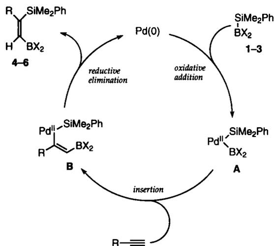
**Scheme 2.** Possible catalytic cycle for palladium-catalyzed silaboration of terminal alkynes (neutral ligands on the palladium atom are omitted).
