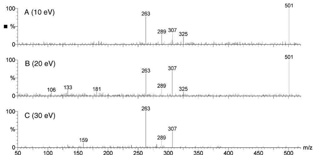
**Figure 6.** HPLC/MS/MS of the main metabolite of gestrinone (Md) generated in ESI+ ion mode at (A) 10, (B) 20, and (C) 30 eV collision energy (daughter ions of  $[M + H]^+$  at  $m/z$  501).
