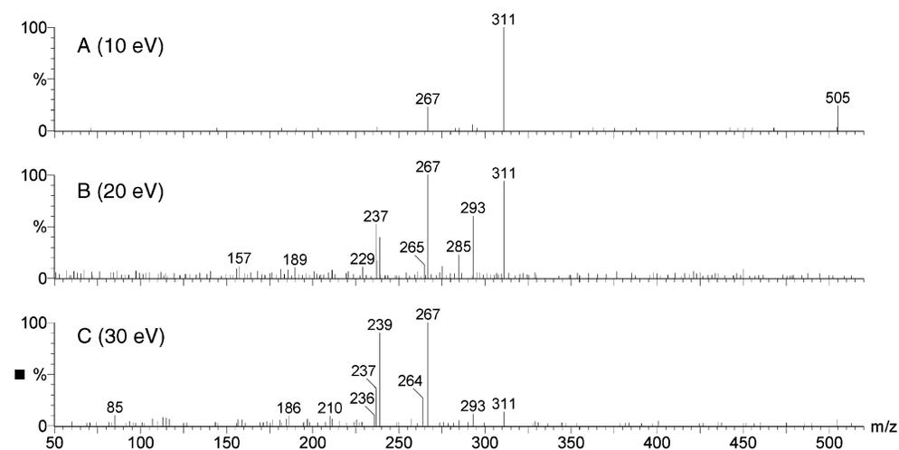
**Figure 4.** HPLC/MS/MS of M2 of THG generated in ESI+ ion mode at (A) 10, (B) 20, and (C) 30 eV collision energy (daughter ions of  $[M + H]^+$  at  $m/z$  505).
