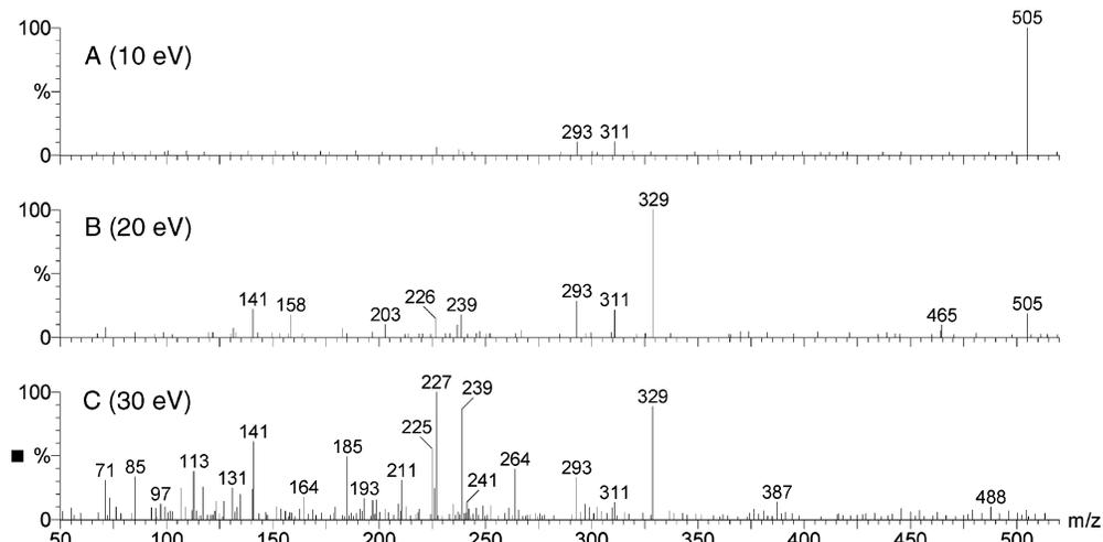
**Figure 3.** HPLC/MS/MS of M1 of THG generated in ESI+ ion mode at (A) 10, (B) 20, and (C) 30 eV collision energy (daughter ions of  $[M + H]^+$  at  $m/z$  505).
