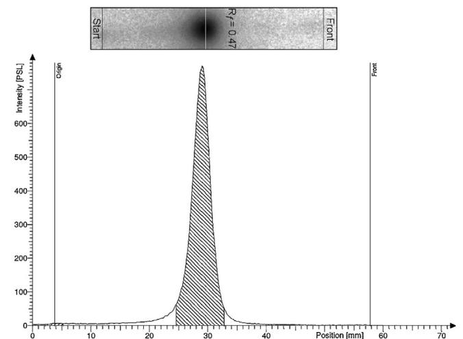
**Fig. 5.** Radio-TLC (eluent: methanol) of [ $^{18}\text{F}$ ]12 after purification using a LiChrolut<sup>®</sup> Si cartridge.
