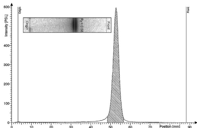
**Fig. 3.** Radio-TLC (eluent: methanol) of [ $^{18}\text{F}$ ]6 after purification using a LiChrolut<sup>®</sup> Si cartridge.
