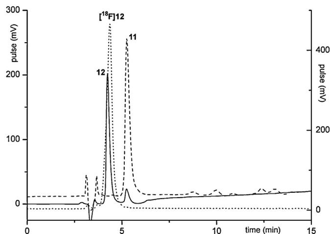
**Fig. 6.** Representative (radio-)HPLC chromatograms from the preparation of [ $^{18}\text{F}$ ]12 (dotted line,  $\gamma$ -trace,  $t_{\text{R}} = 4.4$  min), reference **12** (solid line, UV trace,  $t_{\text{R}} = 4.2$  min) and precursor **11** (dashed line, UV trace,  $t_{\text{R}} = 5.3$  min).
