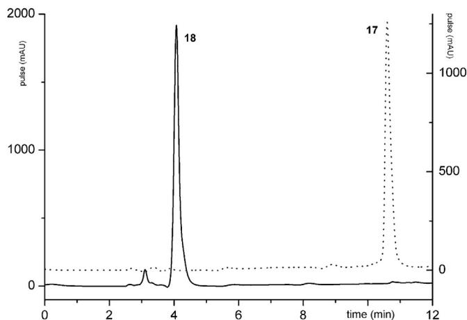
**Fig. 10.** Representative HPLC chromatograms of SNEWILPRLPQH-Azp **17** (dotted line, UV-trace,  $t_R = 10.8$  min) and of the reaction mixture of reference peptide **18** (solid line, UV-trace,  $t_R = 4.1$  min). Gradient: 0 min 10% ACN, 12 min 40% ACN (+0.1% TFA).
