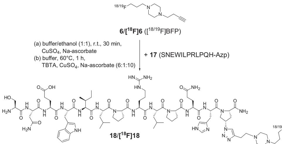
**Scheme 6.** Synthesis pathway to the  $^{18/19}\text{F}$ -labeled peptide **18**/[ $^{18}\text{F}$ ]18 with **6**/[ $^{18}\text{F}$ ]6: (a) Normal conditions and (b) radiolabeling conditions.
