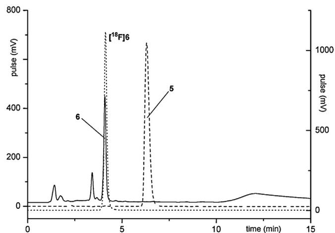
**Fig. 4.** Representative (radio-)HPLC chromatograms from the preparation of [ $^{18}\text{F}$ ]6 (dotted line,  $\gamma$ -trace,  $t_{\text{R}}$  = 4.2 min), reference **6** (solid line, UV trace,  $t_{\text{R}}$  = 4.1 min) and precursor **5** (dashed line, UV trace,  $t_{\text{R}}$  = 6.5 min).
