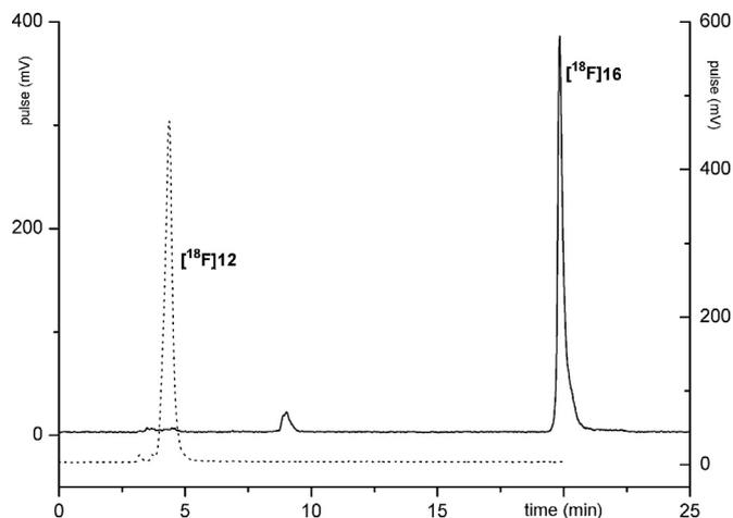
**Fig. 9.** Representative radio-HPLC chromatograms of [ $^{18}\text{F}$ ]12 (dotted line,  $\gamma$ -trace,  $t_{\text{R}} = 4.4$  min) and of radiolabeled amino acid [ $^{18}\text{F}$ ]16 (solid line,  $\gamma$ -trace,  $t_{\text{R}} = 19.8$  min).
