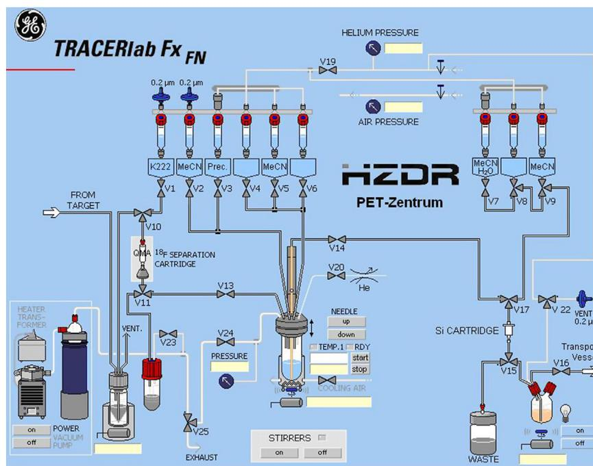
Fig. 2. Scheme of the synthesizer module for the automated radiosyntheses of [<sup>18</sup>F]**6** and [<sup>18</sup>F]**12**.
