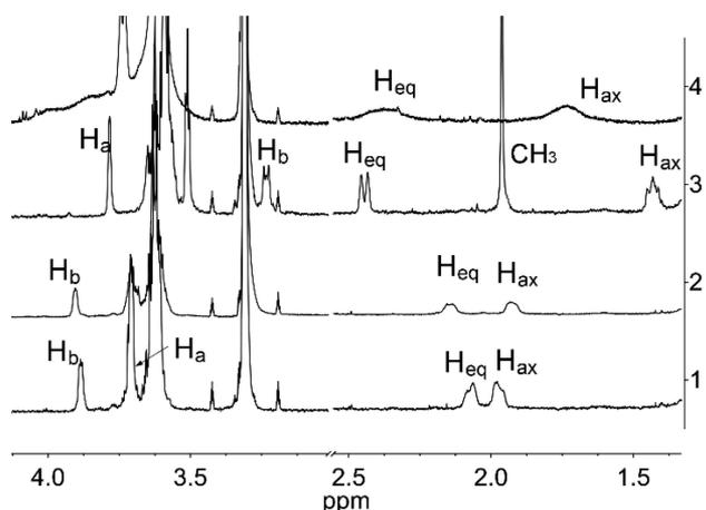
**Figure 2.**  $^1\text{H}$  NMR spectra showing positions of the cyclohexane proton shifts (1) of free receptor **7** in  $\text{CD}_3\text{OD}$ , (2) after addition of 10 equiv of potassium salt to **7**, (3) after addition of 1 equiv of zinc(II) salt to **7**, and (4) of free receptor **7** at  $-60\text{ }^\circ\text{C}$ .
