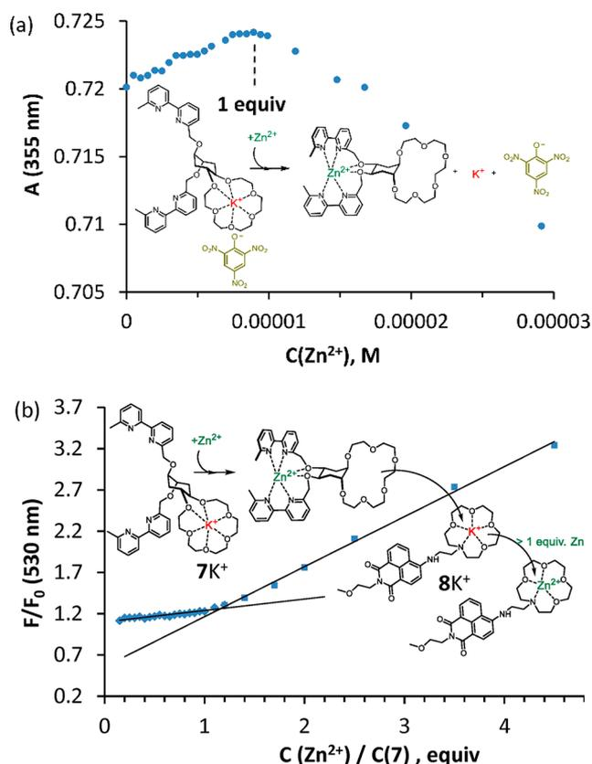
**Figure 3.** (a) Changes in the absorption of picrate induced by addition of zinc(II) perchlorate to a solution of **7** (0.01 mM) and potassium picrate (0.04 mM) in methanol. (b) Changes in the fluorescence spectrum of cation sensor **8** during the addition of zinc(II) perchlorate to a methanol solution of **7** (0.01 mM), **8** (0.01 mM), and potassium perchlorate (0.5 mM). Conditions: ex 440 nm, em 530 nm.
