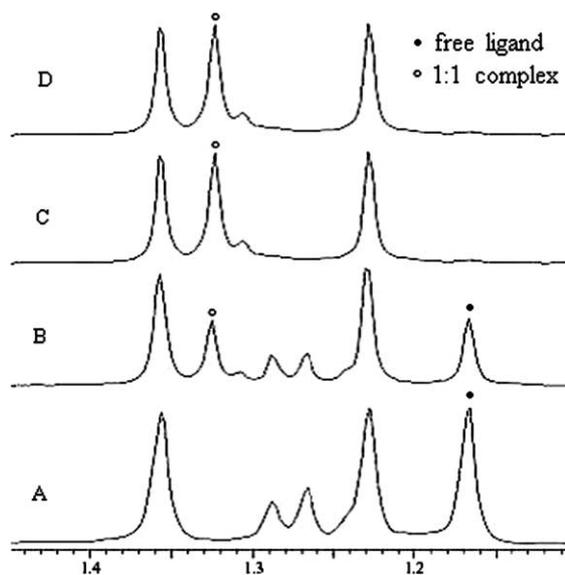
**Figure 4.** *tert*-Butyl region of  $^1\text{H}$  NMR (300 MHz) spectra ( $\text{CDCl}_3/\text{CD}_3\text{OD}$ ,  $v/v = 4:1$ , 298 K) of (A): free ligand **3a**; (B): **3a**+0.5 equiv of  $\text{Cs}^+\text{Pic}^-$ ; (C): **3a**+1 equiv of  $\text{Cs}^+\text{Pic}^-$ ; (D): **3a**+4 equiv of  $\text{Cs}^+\text{Pic}^-$ .
