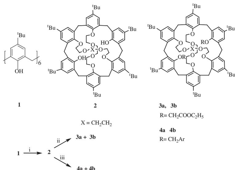
**Scheme 1.** Reagents and conditions: (i) K<sub>2</sub>CO<sub>3</sub>/xylene, triethylene glycol ditosylates, reflux, 12 h, 52%; (ii) K<sub>2</sub>CO<sub>3</sub>/MeCN, ethyl bromoacetate, reflux, 12 h, **3a**, 65%, **3b**, 23%; (iii) K<sub>2</sub>CO<sub>3</sub>/MeCN, benzyl bromide, reflux, 12 h, **4a**, 52%, **4b**, 34%.
