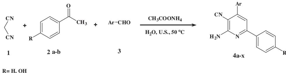
Scheme 1. Synthesis of 2-amino-4,6-diphenylnicotinonitriles under ultrasonic irradiation.
