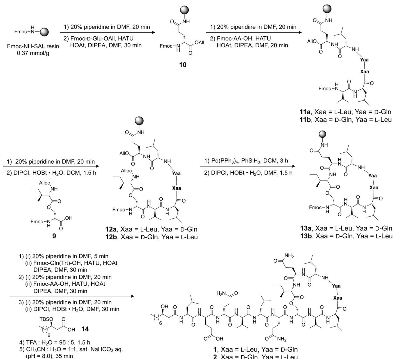
**Scheme 1.** Solid-phase synthesis of MA026 and its analogues. HATU: *O*-(7-azabenzotriazol-1-yl)-*N,N,N',N'*-tetramethyluronium hexafluorophosphate, HOAt: 1-hydroxy-7-azatriazole, DIPEA: diisopropylethylamine, DIPCl: *N,N'*-diisopropylcarbodiimide, HOBT: 1-hydroxybenzotriazole.
