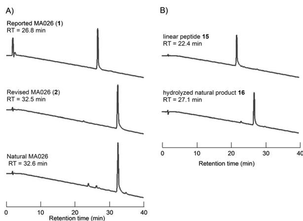
**Figure 2.** HPLC charts of A) reported MA026 (**1**), revised MA026 (**2**) and natural MA026, and B) synthetic linear peptide **15** and hydrolyzed natural product **16**. HPLC conditions: a linear gradient starting from 30 to 70% CH<sub>3</sub>CN in aqueous TFA over 40 min at flow rate of 1.0 mL min<sup>-1</sup>, UV: 220 nm.
