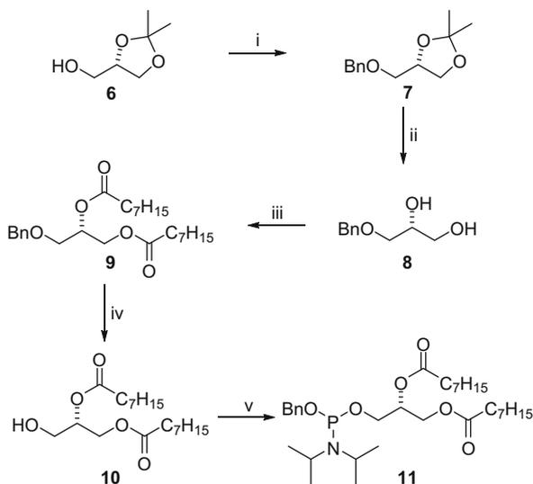
**Scheme 2.** The synthesis of the lipid amidite fragment **x**. Reagents and conditions: (i) NaH, BnBr, DMF, rt, 92%; (ii) concd HCl, MeOH, reflux, 96%; (iii) DMAP, pyridine, octanoyl chloride, rt, 92%; (iv) Pd(OH)<sub>2</sub>, H<sub>2</sub>, THF, rt, 87%; (v) benzyloxybis(*N,N*-diisopropylamino)phosphine, 1*H*-tetrazole, CH<sub>2</sub>Cl<sub>2</sub>, rt, 71%.
