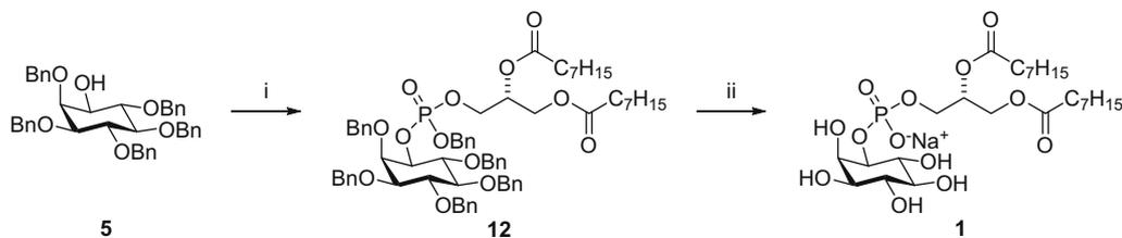
**Scheme 3.** The synthesis of PtdIns **1** by coupling of fragment **5** with fragment **11** and subsequent hydrogenolysis. Reagents and conditions: (i) (a) **11**, 1*H*-tetrazole, CH<sub>2</sub>Cl<sub>2</sub>, rt; (b) *m*CPBA, –78 °C → rt, 52%; (ii) Pd black, H<sub>2</sub>, NaHCO<sub>3</sub>, <sup>t</sup>BuOH, H<sub>2</sub>O, rt, 64%.
